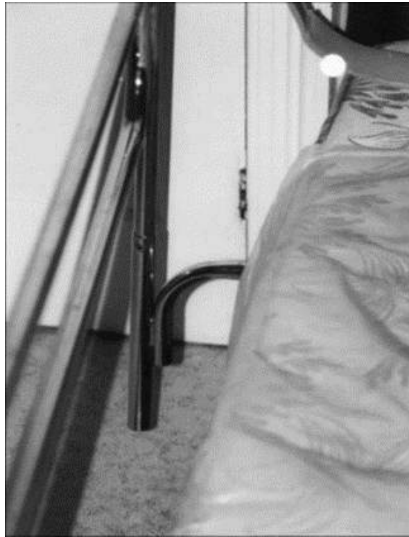
Bed safety rail separated from the bed leaving a gap.
