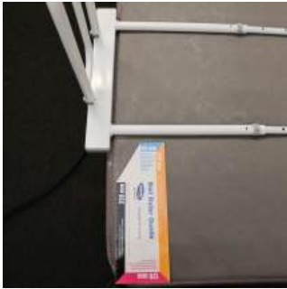
Rail Ruler Guide being used to measure gaps
