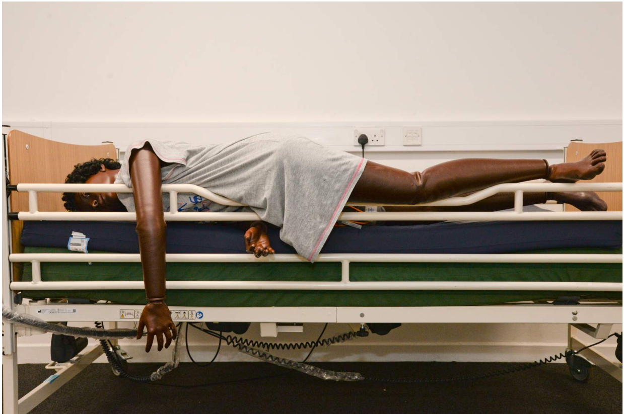
Demonstration showing the reduced height of a safety rail due to the additional height
